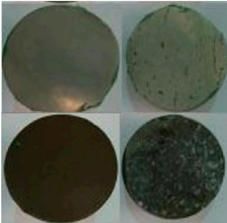
CHEMEON pretreated & coated (top), hexavalent chromated (bottom) AZ-92A-T6 magnesium alloy before (left column) and after (right column) 4 h salt spray testing performed in accordance with ASTM B117.
