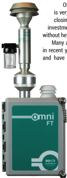
Ambient Air Sampler monitors Cr(VI) Hexavalent Chrome Emissions in Southern California. OmniFT photo used courtesy of Mesa Laboratories, Inc. (Chemeon TCP-HF)
