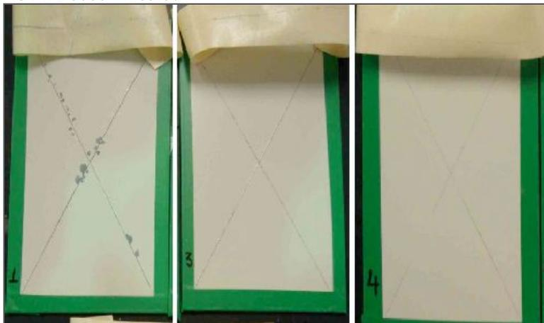
**Figure 6** - Wet-tape tests on non-chromated epoxy primed Zn-Ni plated steel after 168 hr of salt spray exposure: Bare Zn-Ni plated steel (left), hexavalent chromated (center) and trivalent chromium-sealed (right).
