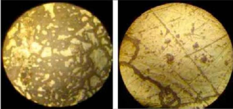
**Figure 2** - Optical microscopy images for uncoated (L) and trivalent chromium conversion coated (R) AZ31B-H24 magnesium alloy surface after 26 hr of exposure to 5% NaCl solution (pH 6.5-7.2) at room temperature.
