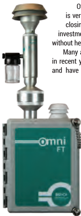
Ambient Air Sampler monitors Cr(VI) Hexavalent Chrome Emissions in Southern California. OmniFT photo used courtesy of Mesa Laboratories, Inc. (Chemeon TCP-HF)
